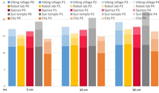
Fig. 13. Runtime of TR for various scenes and viewcell sizes  $|\Delta|$ , reported in ms, broken down by algorithm phase, where P0 is octree layer computation, P1 is geometry generation (which includes the layer-to-layer synchronization overhead), P2 is geometry rasterization, P3 is occlusion interval resolution, and P4 is PVS harvesting.
