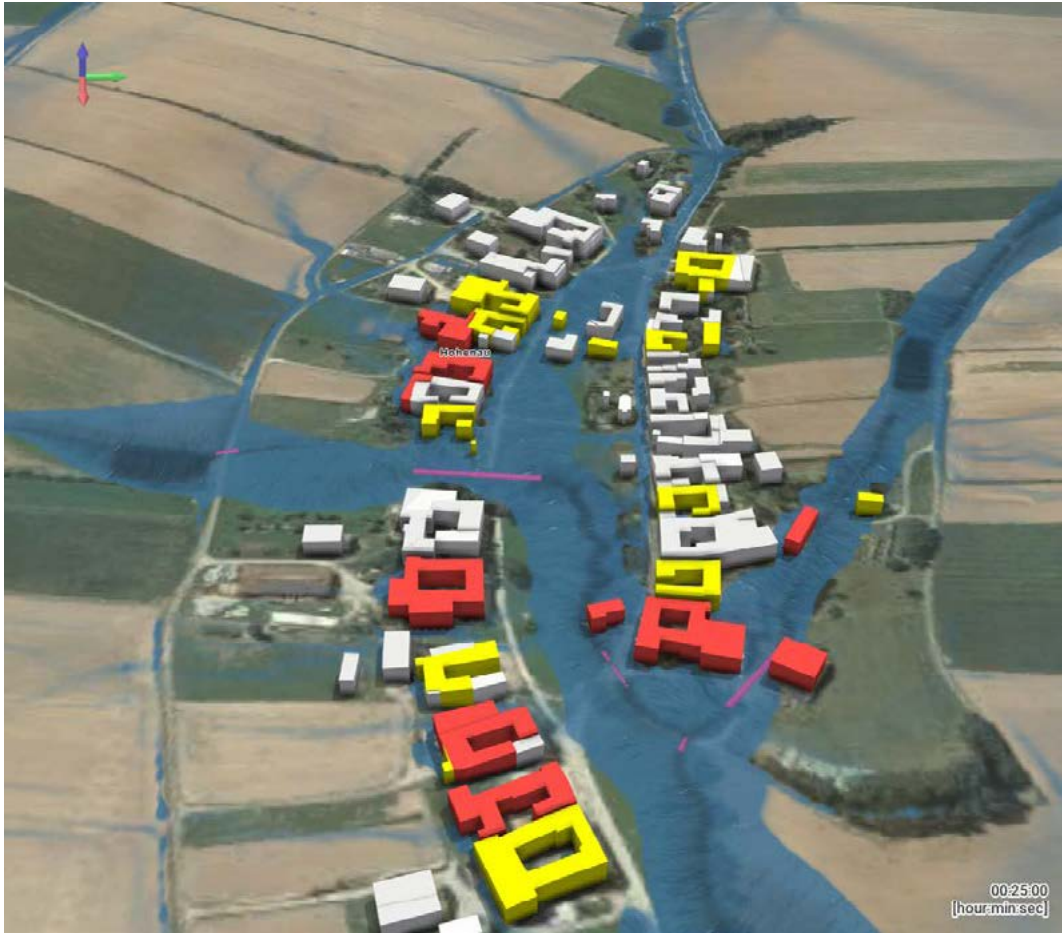
Figure 1 Example of pluvial flooding (shown in blue colour) in the village of Hohenau, Dobersberg after 50mm of rainfall in 15 minutes; building colour shows max. water depth: yellow = min. 50cm; red = min. 100cm
