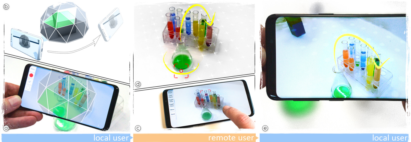
Figure 2. Overview. (a) Scene capture: The local user shares the environment by capturing a local light field. The sampling process is visually guided by a 3D sphere that surrounds the object of interest. The sphere color encodes the current sampling density per subtended angle, allowing to identify those regions of the light field that require more sampling. The target sampling density is automatically specified by the system but may be adjusted by the remote user on demand. (b) Scene exploration: The remote user explores the light field using image-based rendering techniques. (c, d) Scene annotation: Once a suitable viewpoint has been reached, the remote user places a plane in 3D and starts annotating it with drawings sketched on the touchscreen of the mobile device. (e) AR visualization: The visual instructions are sent to the local user and presented within the 3D coordinate system that was used for capturing the light field. Therefore, the visual instructions naturally appear as 3D-registered augmentation in the local user's environment.
