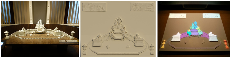
Fig. 1. From left to right: a) The table fountain as displayed in the museum. b) Realistic rendering of the final tactile relief design. c) Produced tactile relief CNC milled from DuPont Corian® used in our interactive audio-guide with projected colors indicating interactive regions.
