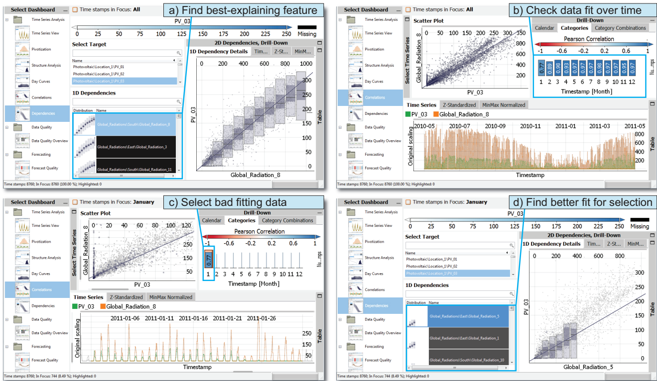
Figure 2: Example dashboard workflow to model photovoltaic power production. The analyst first starts the dashboard 'Dependencies' and selects the best-explaining feature for power plant 'PV_03': Global.Radiation_8 (a). She switches to the 'Correlations' dashboard and discovers that for January, the goodness of fit is significantly lower compared to the rest of the year (b). She selects January (c) and switches back to the 'Dependencies' dashboard. She discovers that for the selected data, 'Global.Radiation_5' is a better fit (d). To optimize model performance, she considers creating a composite model for 'PV_03' involving both 'Global.Radiation_5' (January) and 'Global.Radiation_8' (rest of the year).
