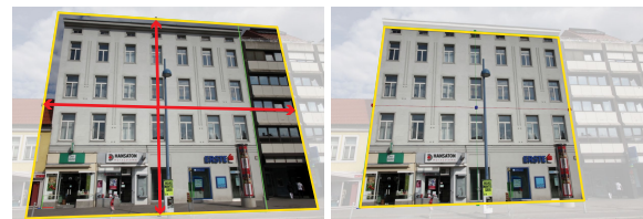
Figure 4: View at the façade plane through one of the projecting cameras. In this view it is easy to adjust the façade-bounds interactively. Left: during the adjustment. Right: final result.
