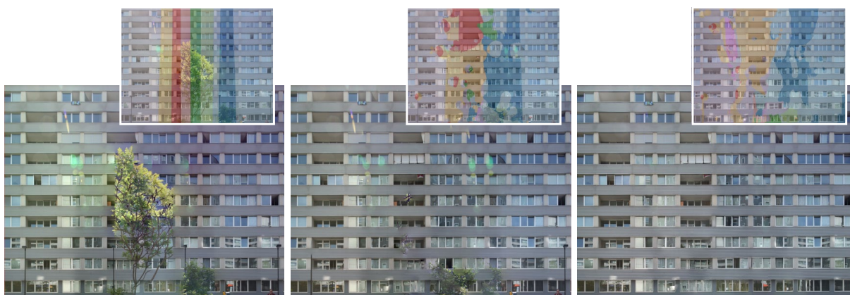
Figure 12: Automatic removal of occluding objects by utilizing the information from structure-from-motion points. Left: image and its mask after multi-view stitching without the occlusion term. Middle: results with occlusion term. Right: result with occlusion term post-processed by interactive brushing. Note that lens flares have been removed as well.
