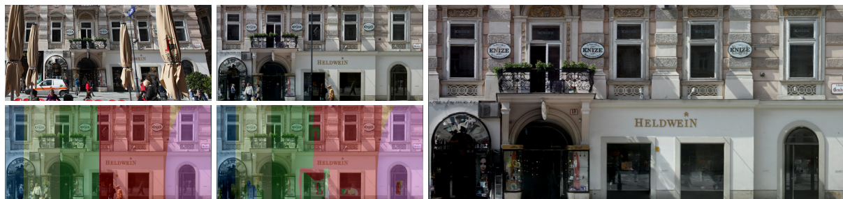
Figure 1: Steps of the proposed multi-view image generation system. Top-left: one of typical perspective input photographs, please note the occlusion. Top-middle: the result of the proposed ortho-image generation method (note the pedestrians). Second row shows masks indicating source images of the composition by colors: automatic result (left) and interactively post-processed (middle). Right: the final result after interactive post-processing.
