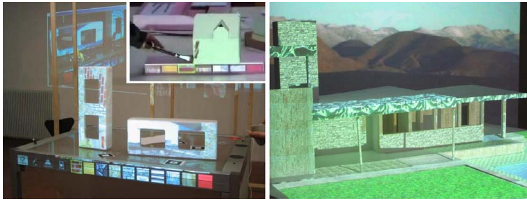
Figure 10. (left) configuring the Texture Brush for painting a model, on the border of the table, the menu bar, (right) a painted model from two directions with background.
