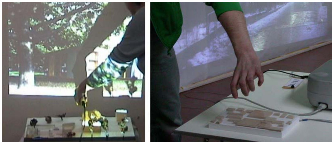
Figure 4. a) barcodes placed onto models, b) touch sensors integrated into model
