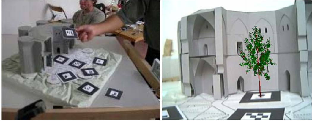
Figure 11. Using optical markers for inserting a virtual tree into a physical model
