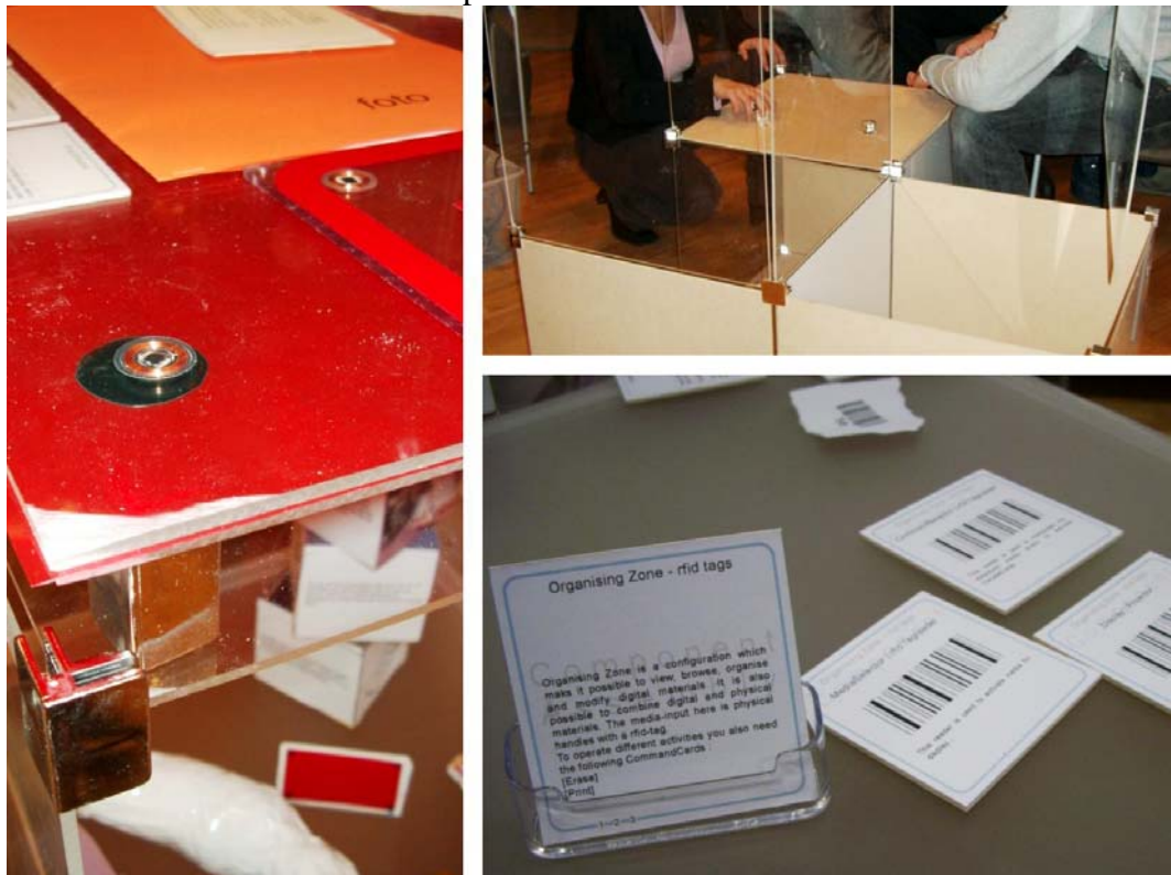
Figure 8. Tag reader integrated in the furniture (left); building different forms of furniture with modules (up right); the configurator deck of cards (down right)
