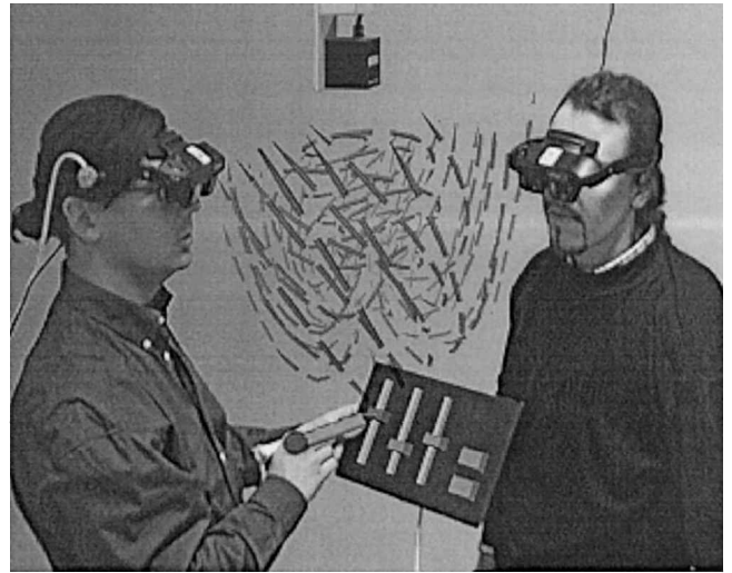
Figure 1. Two collaborators wearing see-through displays are examining a flow visualization data set.
